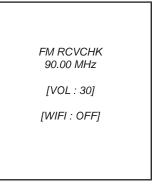
90.00 MHz (default)  $\rightarrow$  76.00 MHz  $\rightarrow$  95.75 MHz  $\rightarrow$  107.75 MHz  $\rightarrow$  87.50 MHz  $\rightarrow$  98.00 MHz  $\rightarrow$  108.00 MHz
